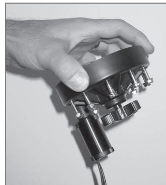
Diaphragm support ring prevents stress failures.
